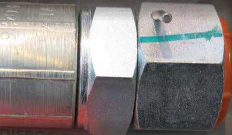
Thrust-wire protruding from termination end
