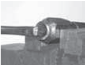
Apply lubricant to stem and hose tube.
