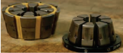
Always verify proper die set. Insert die set in crimper.
