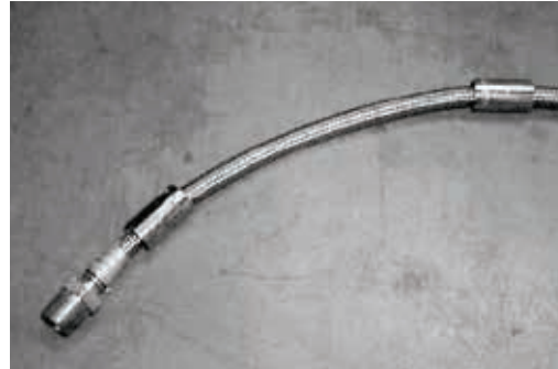
Hose with attached ferrules.
