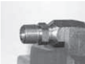
Stem properly seated against socket.
