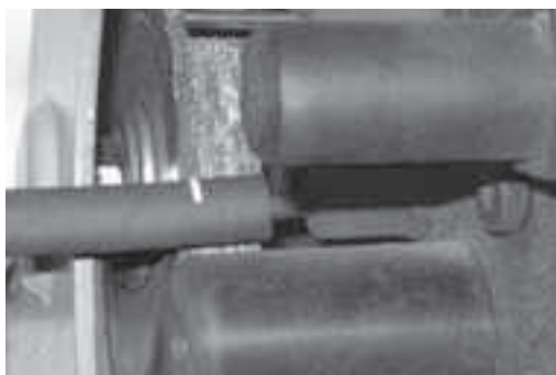
Cutting skive with buffing wheel. Follow manufacturer recommendation for the safe and proper use of the skiver.
