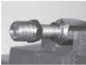
Screw stem into socket.
