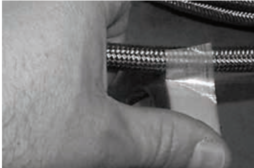
Tape hose before cutting.
