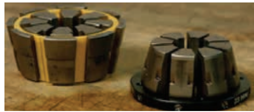
Always verify proper die set. Insert die set in crimper.
