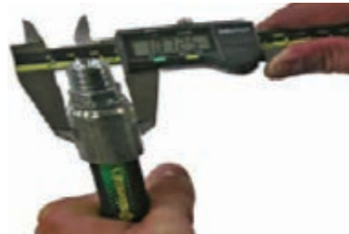
Verify crimp diameter with calipers.
