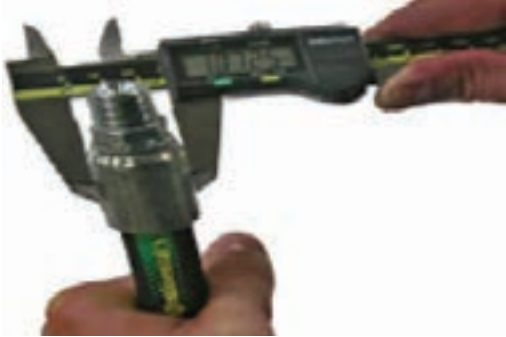
Verify crimp diameter with calipers.
