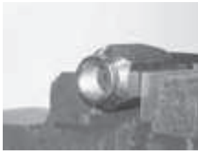
Visually check hose position inside socket.
