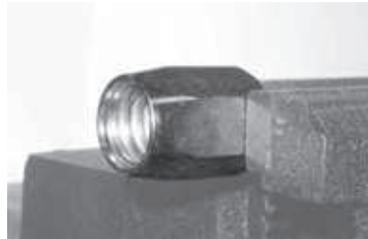
Socket positioned in vice.
